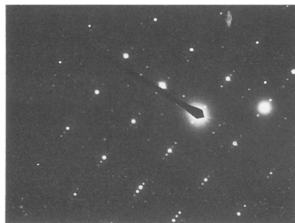
Figure 4 Electron diffraction pattern of superconducting \text{BiSrCaCu}_2\text{O}_x phase.
