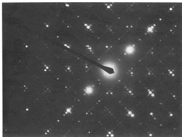
Figure 5 Electron diffraction pattern showing the presence of microdomains in \text{BiSrCaCu}_2 -oxide.
